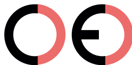
False CE Mark (too far)
